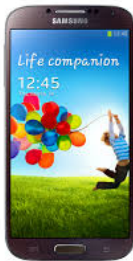
Figura 4.5: Smartphone Samsung Galaxy S4 octa-core chipset, 1.6-GHz Quad + 1.2 GHz Quad CPU.
